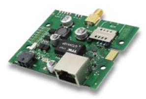
Small and quick to deploy industrial Ethernet to 4G LTE IoT gateway. Advanced VPN functionality, security and remote management capabilities makes TRB140 the best option for single device connectivity.
